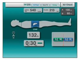
Input your date once, and from there the alpha7 will calculate the injection rate automatically. Just selecting an anatomic region,the alpha7 can calculate the contrast media volume required for your protocol.
